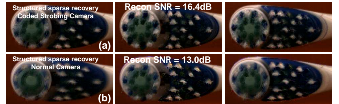
Fig. 14: Reconstruction results of toothbrush with upsampling factor U = 50 . Note that using CSC to capture periodic scenes allows us better reconstruction over using a normal camera.
